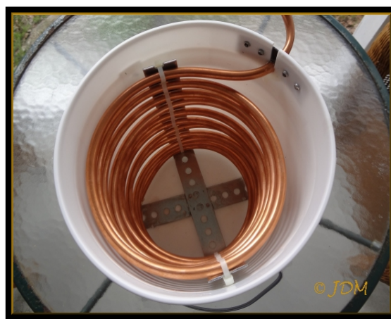
Fig. 18: Inside of a constructed desalination kit
